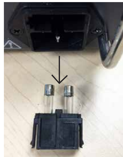
Figure MM-02 Fuse Holder Removed
