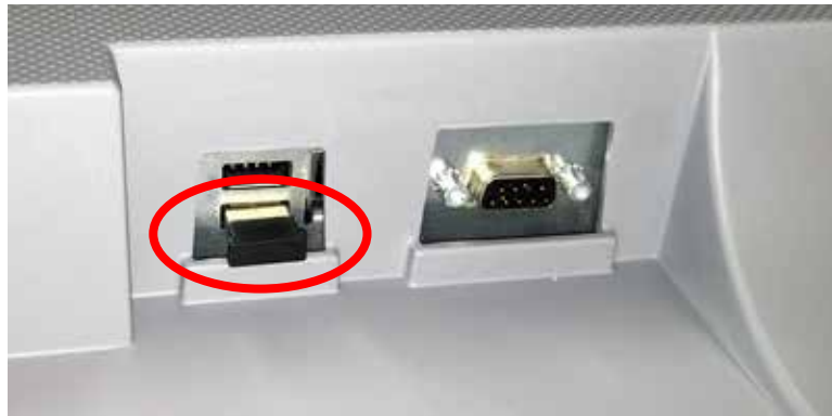
Figure IS-22 Bluetooth Installed
