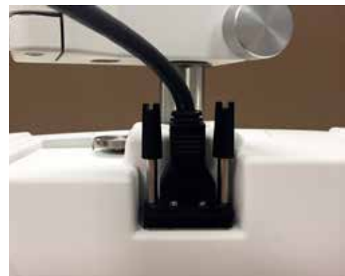
Figure IS-09 Cable Installed
