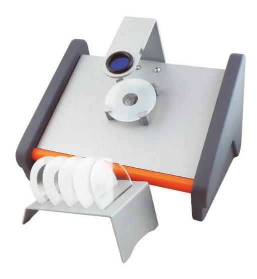
The device consists of a housing and a forehead support. A patient leans the forehead and observes through the magnifying glass the Haidinger phenomenon used in this device.
