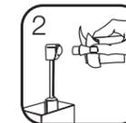
Insert the tip into the tonometer with the line aligned to the zero position.
